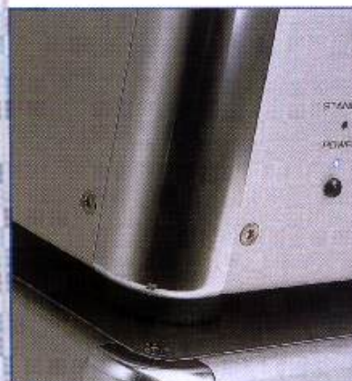
The brushed aluminium panels are fastened by rounded chrome-edge caps
